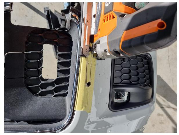
30. Using a jigsaw or other cutting tool, cut out the area marked.
