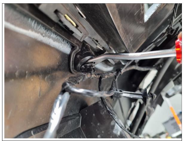
28. Unclip the loom behind the marked area and secure to the side and out of the way with cable ties.
