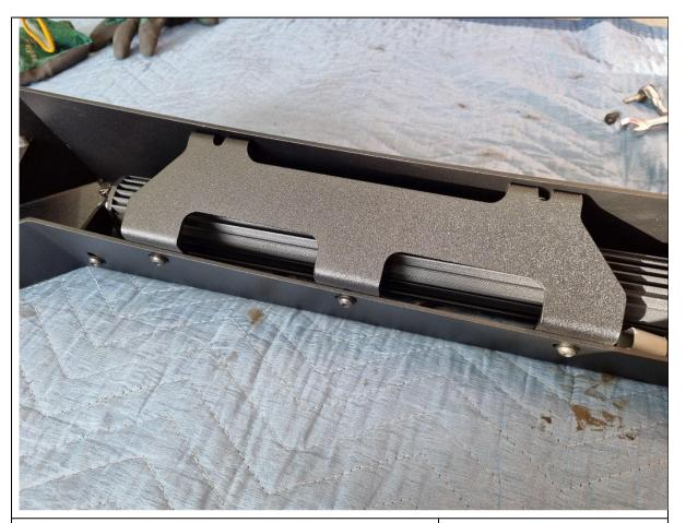
39. Fit the 2x Tactical Nudge Bar centre gussets to the back of the Tactical Nudge Bar, using 5x M6x16 black button head bolts, black flat washers and flange nuts on each gusset.
