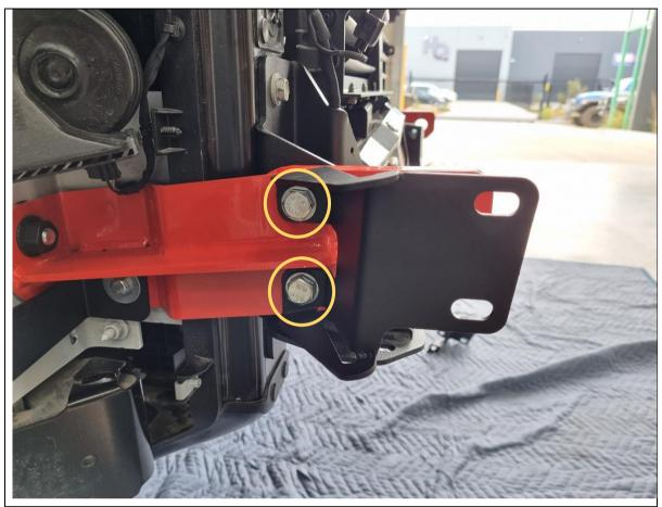
25. If using the Offroad Animal Recovery Points, bolt the nudge bar chassis bracket to the outside of the recovery point using the provided M12x55 hex head bolts, washers and nuts. Do this on both sides.
