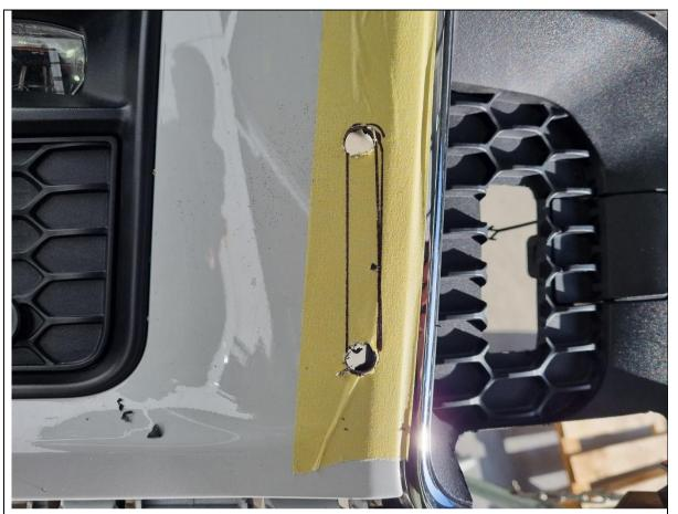
29. Use a 10mm drill bit and drill 2x holes at each end of the marked slot.
