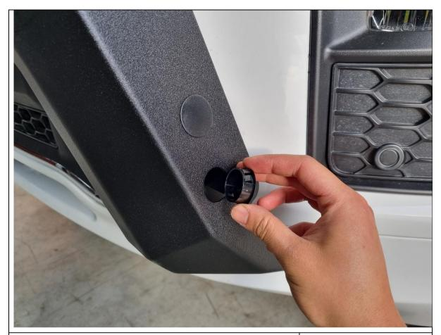
47. For the Tactical Nudge Bar, plug the bolt access holes with the supplied plastic plugs for a sleek finish.
