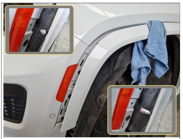
11. Pull and release the clips retaining the flare to the bumper + quarter panel.
